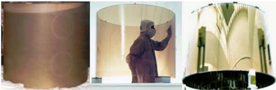
Fig. 1— Chandra mirror elements shown at different stages of production. Left to right: (Left) Glass substrate prior to grinding and polishing. (Center) Fully polished shell being inspected. (Right) Coated shell.
