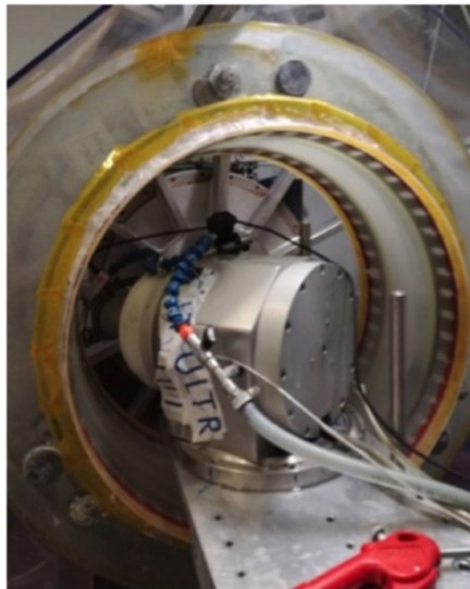
Fig. 5—(Left) A representative shell on the lathe during the grinding process at OAB. (Right) Shell support structure mounted to diamond turning machine at MSFC.
