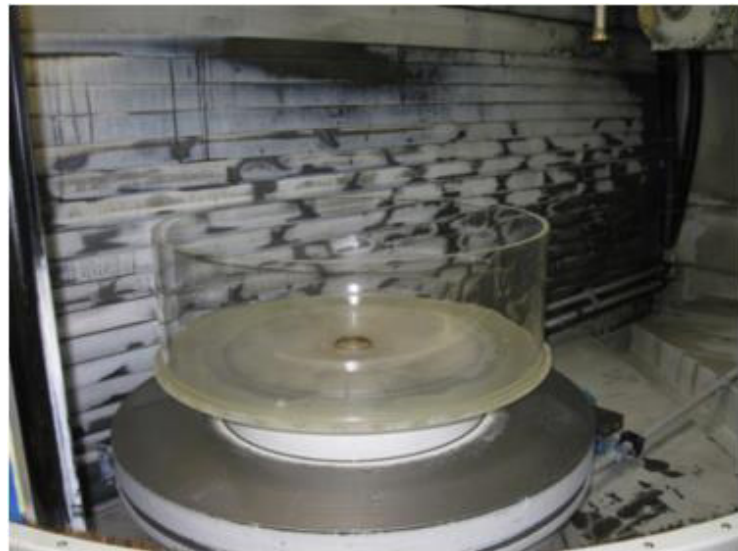
Fig. 4—A cylindrical tube of fused silica before the grinding to generate a double-conical configuration
