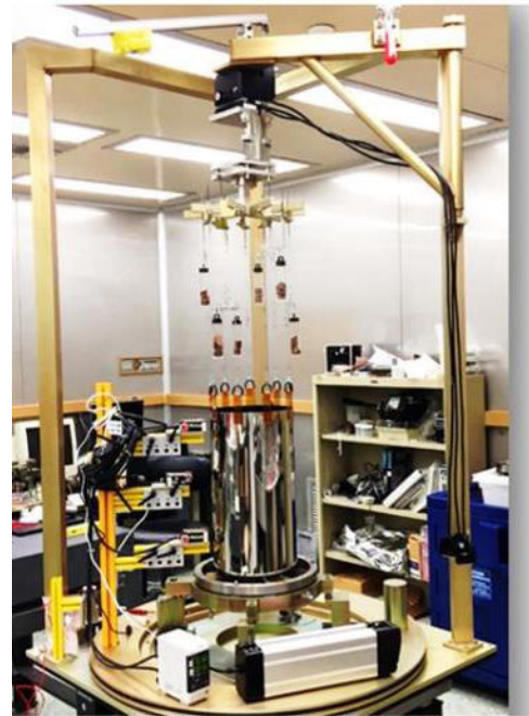
Fig. 9—Hanging wire station for final stage bonding at MSFC.
