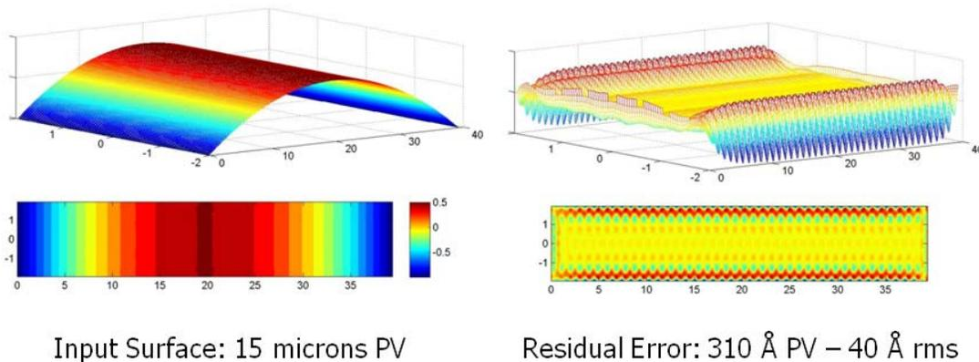
Figure 6. Residual error from actuating a plane surface to the axial figure required of one of the primary mirror reflectors of the Gen-X concept
