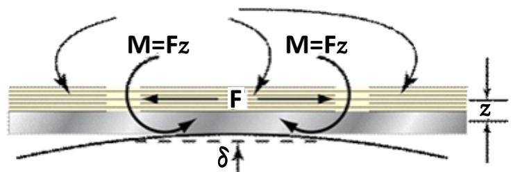
Figure 4. Surface Parallel Actuation Deformable Mirrors
