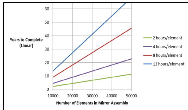
Figure 3. Time to Construct Mirror Assembly
