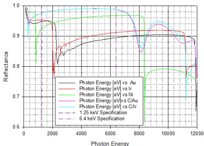
Figure 10. Reflectance vs. Photon Energy for Different Surface Coatings
