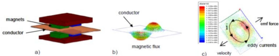
Figure 8. a) Maxwell 3D fine element model of magnetic damper. b) Magnetic flux distribution at the conductor center plane (from magneto-static analysis). c) Eddy currents generated on conductor as it moves at a constant velocity (from transient analysis).
