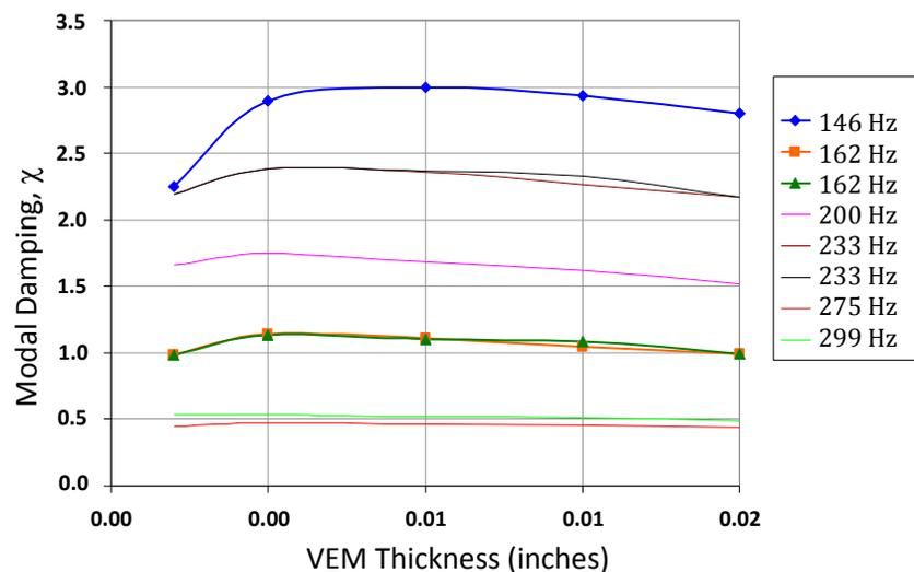
Figure 7. Damping performance vs. VEM thickness. Legend shows original un-damped natural frequency.
