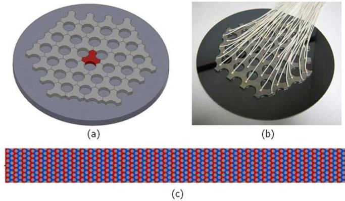
Figure 5. Finite element analysis model (c) and test optic component (b). Diagram (a) shows region (red) that constitutes one actuator within lamellar structure.
